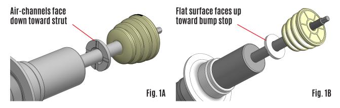
23. For models years 2009-2013, install the supplied 10mm washer and stem sleeve found in hardware kit 25001-778 prior to placing the strut inside the spring and top mount.
