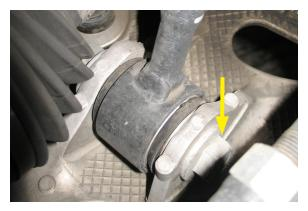
12. Break loose the 21mm outer tie-rod nut but do not remove yet. Strike the tie-rod mount with a dead-blow hammer until the ball joint is dislodged then detach the tie-rod from the spindle.
