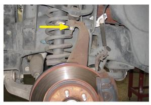
14. Remove the three 15mm top mount nuts. Slide the spring and shock assembly down and out of the front suspension. To help the installation, mark the outboard side of the spring and upper shock mount with a paint pen for reference to the original position.
