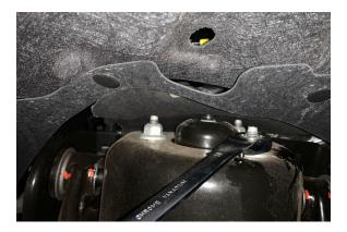
28. Attach the upper control arm ball joint to the spindle. Torque the nut to 85 ft lbs.
