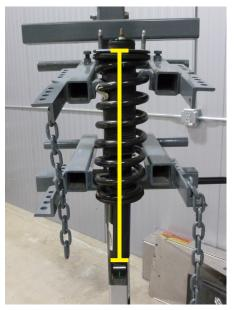
16. Using a 17mm wrench (stock nut size) and a 8mm wrench, remove the top nut from the strut assembly (DO NOT USE AN IMPACT GUN). Remove the top nut and mount. You will use the top mount with your new Belltech strut later.
