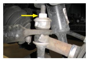
11. Remove the 30mm lower strut mount nut to remove the bolt holding the strut to the lower control arm.
